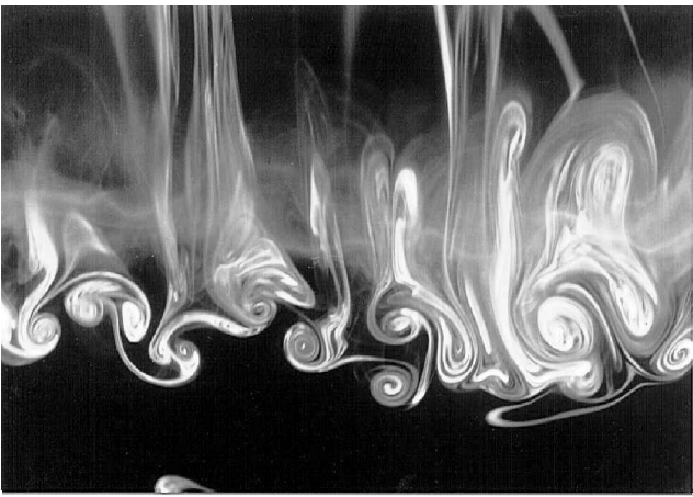
a) Experiment ( Re \approx 2.5 \times 10^3 and t^* \approx 10 ), dye visualization
